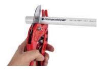
Normally, while cutting the multilayer pipe, the pipe is deformed. The section we made when cutting is elliptical, due to the hardness that the intermediate layer of aluminum offers to the multilayer pipe, which cause a problem when assembling the fittings, since it costs much more to insert these fittings to the pipe.
