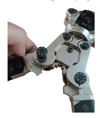
Turn the numerical indicator to the desired position, being the position 1 the slightest and the position 5 the most intense. Insert the numerical indicator till it fits in its place
