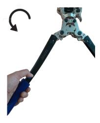
Press using both handles until the stop
