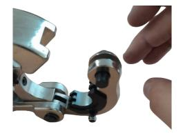
Press the spring-loaded pin
