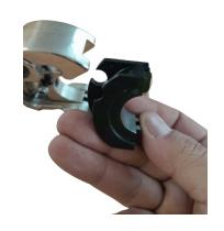
Fit into its position and release the pin
