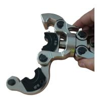
Insert the pipe with the fitting and close the pin
