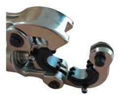
Press the spring-loaded pin
