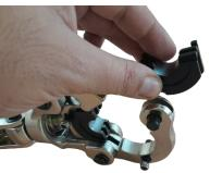
Press the spring-loaded pin to release the clamp
